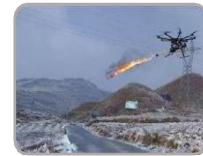
Flame Ice Removal: Small range, poor effect
