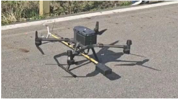
Airborne insulator inspect device
