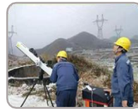
Laser Cannon De-Icing: High power consumption, small range
