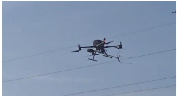
Airborne insulator inspect device take off
