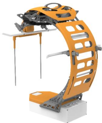
Manually-mounted Insulator Inspect Robot
