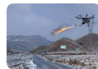
Flame Ice Removal : Small range, poor effect
