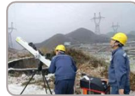
Laser Cannon De-Icing: High power consumption, small range
