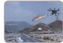
Flame Ice Removal: Small range, poor effect
