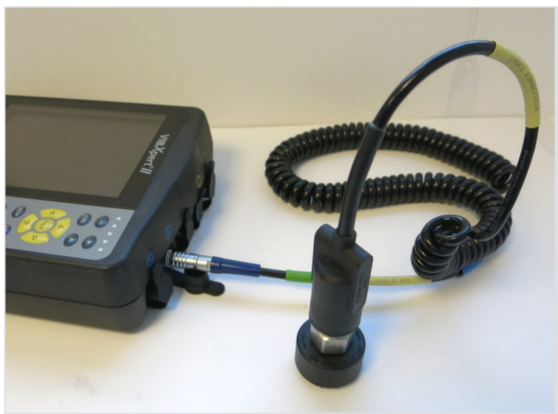
Sensor VIB 6.142 connected to VIBXPERT II using the spiral connection cable VIB 5.436
