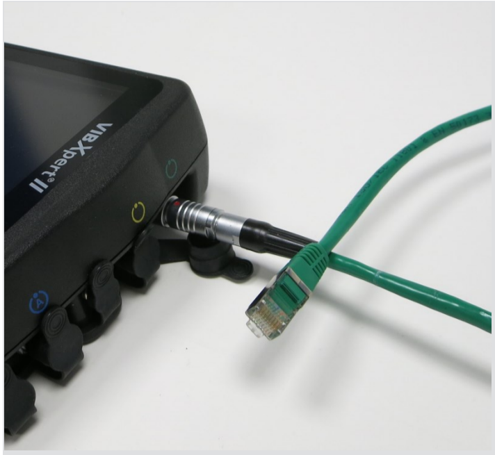
Ethernet cable connected to VIBXPART II
