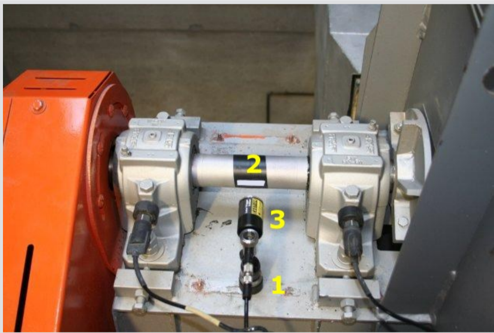
Measuring RPM: Stand (1), the reflective tape is on the shaft (2) and RPM sensor (3).
