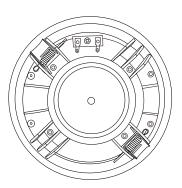
The FYB Active Bluetooth In-ceiling Speaker designed with digital Class D amplifier and utilization of 6W dual-cone dynamic speaker driver, will provide a clear and warm sound and suitable for installation in almost any material. Ideal for use in your living room, bedroom, hotel room, entertainment area, office, workspace, showroom, restaurant etc.
