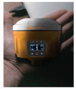
The highly integrated four-in-one antenna on the M7 provides several advantages, including saving space, improving performance and reliability, and reducing the failure rate during use, making M7 more portable and easier to handle, increasing the efficiency and accuracy of measurements.
