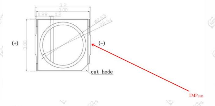
The recommended Ts point is located in the bottom of PCT3030
