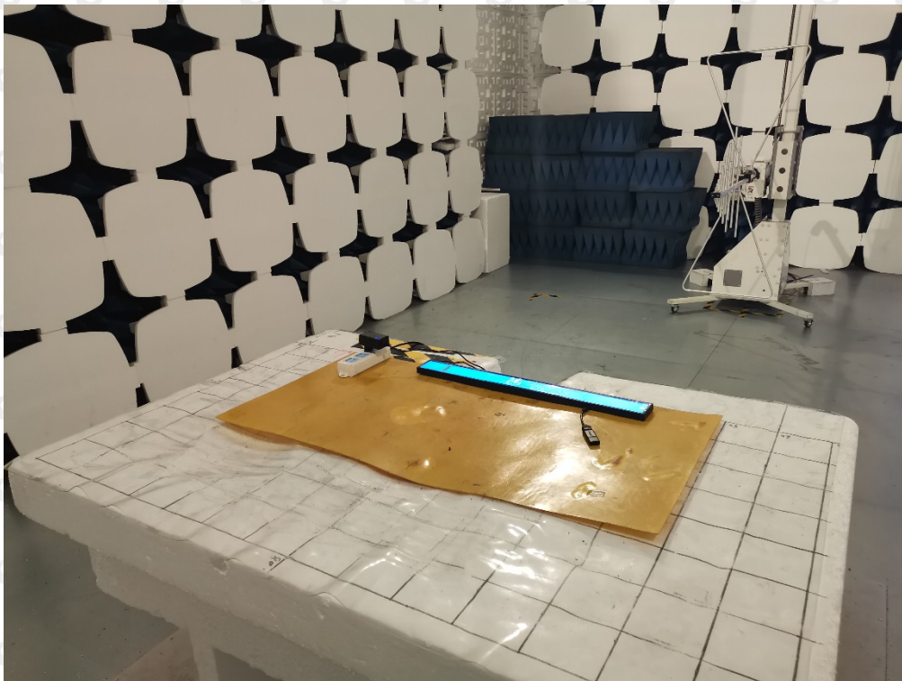
Photograph of test setup for Radiated Emission
