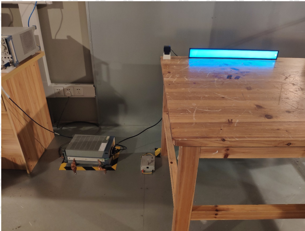
Photograph of test setup for Conducted Emission
