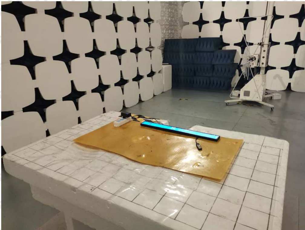
Photograph of test setup for Radiated disturbance
