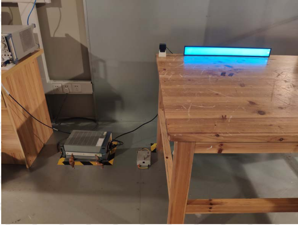
Photograph of test setup for Conducted Emission
